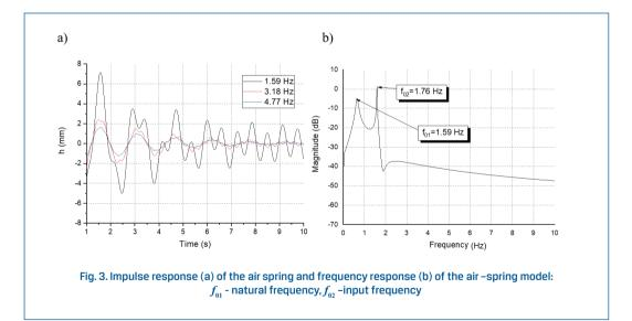
In the simulation system of the bellows actuator model, a decrease in amplitude is observed in the natural frequency range  $f_{01}$  as well as in the original input frequency range  $f_{02}$ . The natural frequency of the mechanical system was determined by the Fast Fourier Transform (FFT) (Figure 3b) from the impulse response (Figure 3a).
