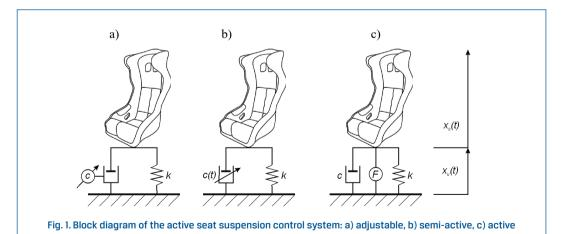
In this type of suspension, the damping and elasticity coefficients are adjusted to the prevailing operating conditions [4]. Many constructions use solutions that allow the operator to change the damping coefficient c depending on the individual assessment of operator's weight and operating conditions (Figure 1a). Effective damping can be achieved automatically or manually by setting a default pressure (pneumatic spring) or tension
