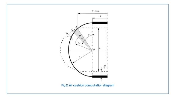
Assuming that the distance of the mass centre for an elementary triangle is in 2/3 of its height and applying Pappus's centroid second theorem, the total volume of the air cushion after deflection can be determined according to the formula:
