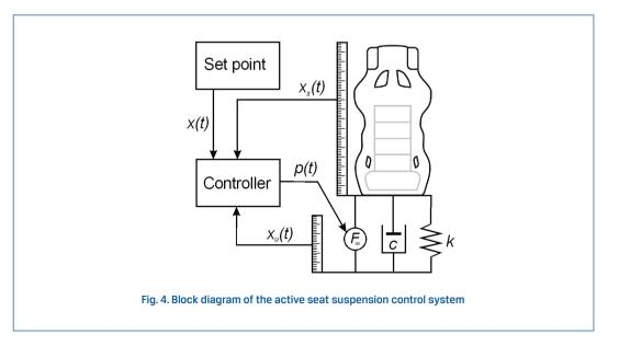
The role of the controller is to adjust the pre-set pressure in the bellows actuator to minimize seat acceleration. The initial bellows pressure determination depends on the vibration-insulated mass. The Fas force generated in the active system depends on the control signal or on the current seat deflection  $x_u$ - $x_s$  which is the measured value.
